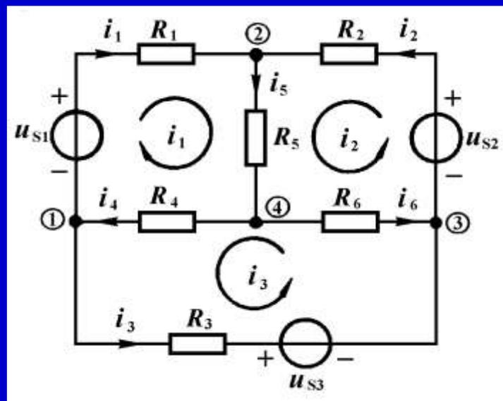
$$\left. \begin{aligned} R_1 i_1 + R_5 i_5 + R_4 i_4 &= u_{S1} \\ R_2 i_2 + R_5 i_5 + R_6 i_6 &= u_{S2} \\ R_3 i_3 - R_6 i_6 + R_4 i_4 &= -u_{S3} \end{aligned} \right\}$$
